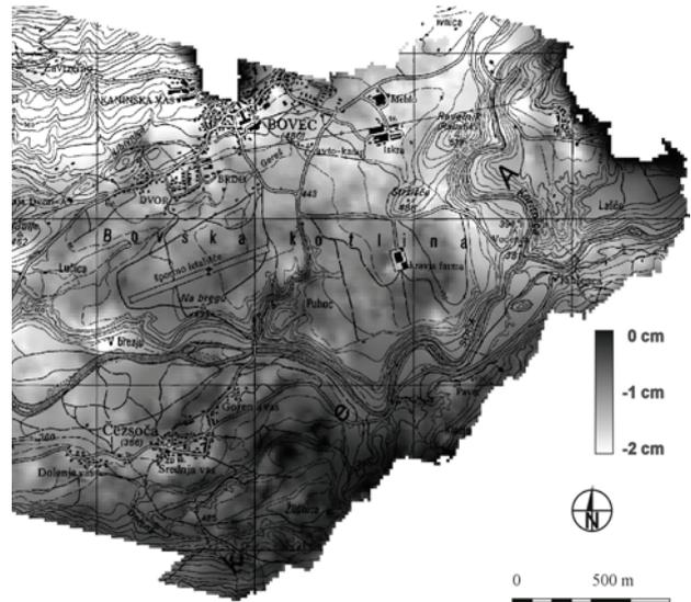
Fig. 6 Displacement caused by earthquake [6].
