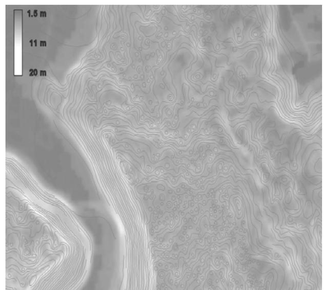
Fig. 2 Surface of predicted random error for a reference DEM (denoted as  $RU$ ), with contour lines.
