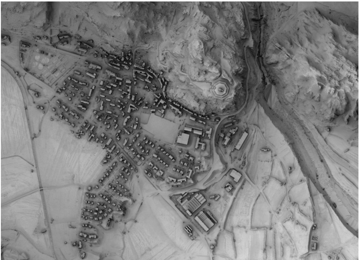
14) Advanced analytical shading: A comparison of classical (a) analytical shading and (b) one of the options applying the multidirectional visibility index (MVI) (below, Podobnikar 2012). The data source is a lidar digital surface model (DSM) with a resolution of 1 m. (small town Kobarid, NW Slovenia) (2012).
